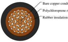
Bare copper conductor Polychloroprene rubber outer jacket
